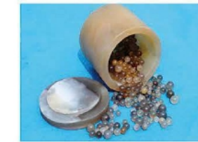
Agate mill pot can be matched with agate balls
