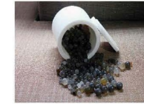
PTFE mill pot can be matched with agate balls
